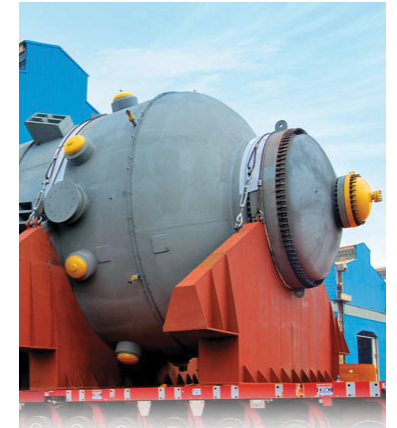
WORLD'S HEAVIEST FCC Regenerator
